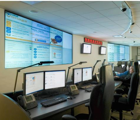
DLP cubes fall somewhere in the middle in terms of cost, with a lifespan, in Mitsubishi's case, of up to 100,000 hours, which is over 11 years of continuous service. This is a proven technology intended primarily for the control room, and issues with maintenance and spare parts are rare. For those reasons, cubes remain the first choice for nearly all mission-critical control rooms, especially those used 24/7/365.
