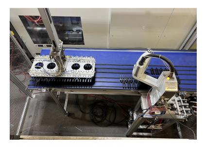
"First, the robot is able to create a much straighter stack of shims, coming out of the heat sealer, than operators were able to achieve by hand. "The people at Glazelock really like the new appearance of the shim stack; it sets their product apart from their competitors," Allen explained.
