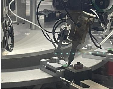
These meters are small assemblies with a one-inch diagonal LCD display that notify users when it's time to change the oil and perform other necessary maintenance. "We are soldering a tiny piece of metal onto a printed circuity board, and that must be done in a very accurate manner," McArthur explains.
