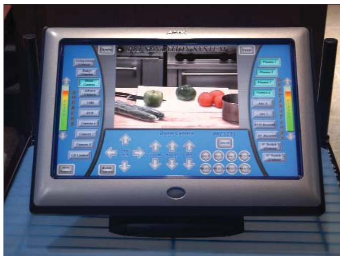
Media Resources used a 17-inch AMX Modero touchpanel control system to make the AV system easy for instructors to navigate
