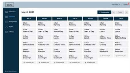
**#ES.** The Bodhi Event Scheduler combines a calendar with a job panel to create and schedule one-time or recurring events using almost any kind of technology. For example, turn lights on or off and select lighting levels. Combine multiple fixtures into groups and schedule them together. Set up or trigger presets and scenes. Schedule by the hour and minute or by the astronomical times of sunrise and sunset.
