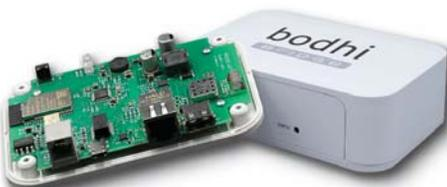
The Bridge combines a wireless radio with an Ethernet port, two wired general purpose inputs, and either a Wi-Fi or LTE cellular card. Together they allow you to connect up to 32 certified Bodhi wireless devices plus water meters, AC power meters, and specialized instruments and sensors to Bodhi.
