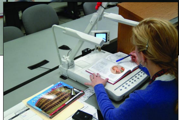
This Latin language class originates at Payton but includes students from Von Steuben High School. The distance learning system includes three robotic cameras, four Pioneer plasma displays and an operator's station with source equipment, codec and controls (shown on cover). Instructors use the document camera in place of a blackboard (see photo at right).
