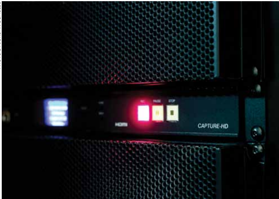
Currently installed at OSU, Crestron Capture HD captures a 1080p, 24 frames-per-second signal.
