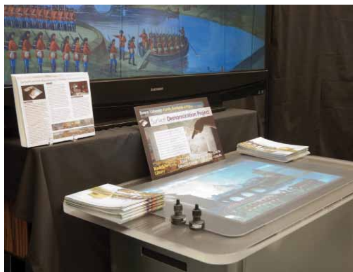
The original Microsoft Surface demonstration unit, with its 30in. touchscreen and a section of the Garibaldi panorama on display. The finished system uses two 50in. Panasonic displays with DualTouch overlays and Windows 8 for touch support.
