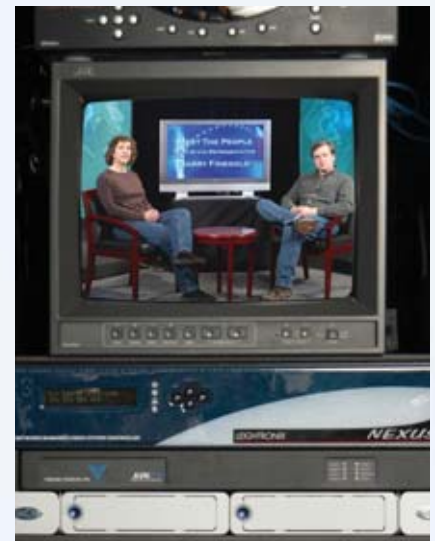
The Nexus video server and VSI encoder in AndoverTV's studio rack
